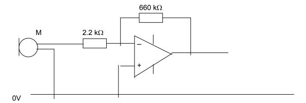
Non-inverting input (+) connected to 0V line (1)
